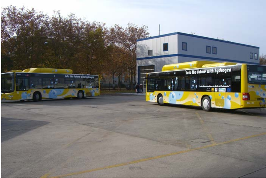
Hydrogen Buses on the service point of BVG in Berlin; Left: Bus with aspirated engine Right: Bus with turbo charged engine; At the background: Maintenance building for Hydrogen Busses
